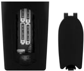
Figure 18 – Remote Battery Compartment
